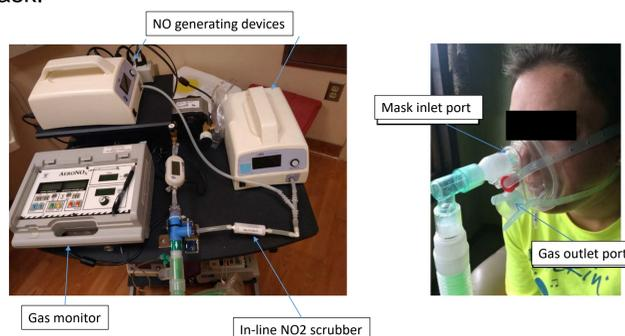
Fig. 1. Inhaled NO Delivery System
